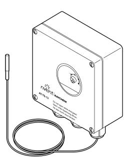
nVent RAYCHEM AT-TS thermostats provide temperature control in safe area. The temperature set point can be checked through a window in the lid. LED's are providing an indication when cables are energized (Heating ON) or when the temperature sensor is defect (sensor break or sensor short-circuit).
